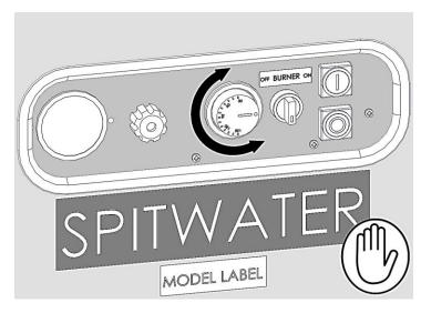
3. After hot water use, turn burner switch in anticlockwise to turn OFF the hot water and change back to cold water mode for cleaning.
