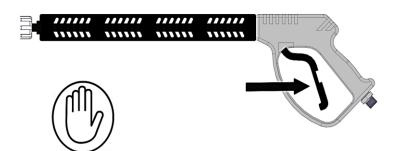
Check that the pressure indicated on the pressure gauge matches the value on the data plate and in the technical data. Also check that when the trigger is released the pressure shown on the gauge returns to zero.
