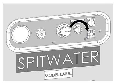
2. Turn the temperature adjustment knob to achieve desire cleaning temperature.
